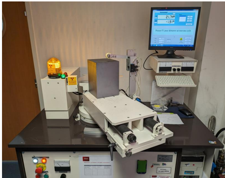
Figure 6: Goniometer equipment (CEA) – (110) plane misorientation measurement
