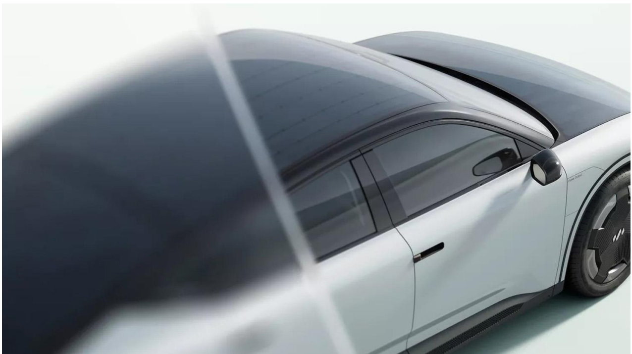
Figure 4-21: PV cells integrated in LEV (source: TNO)
